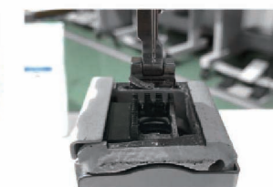
Upper and lower feeding facilitates heavy materials Zigzag model. ※ ST-2452/3
